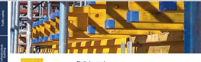
3-layer shuttering panels, glued in itself, with longitudinal running outer layer and transverse middle layer, the wood is aligned with the outer layers to avoid cracks, the gluing carried out with melamine-formaldehyde resin (MUF) according to SWP/3, external condition of the standard UNE CEN/TS 13353, which ensures a high
