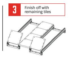
Continue the process to desired width. Use FOUNDATION connectors to join sections end-to-end to desired length.
